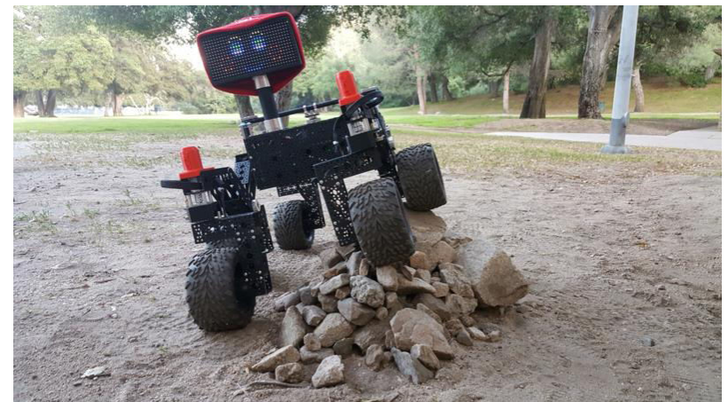
NASA Open Source Rover powered by a Raspberry Pi 3
